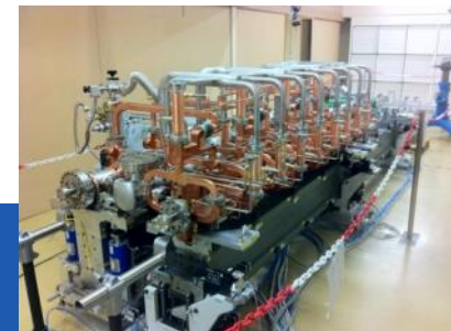
Various RF elements of a complete module, X-band test stand
